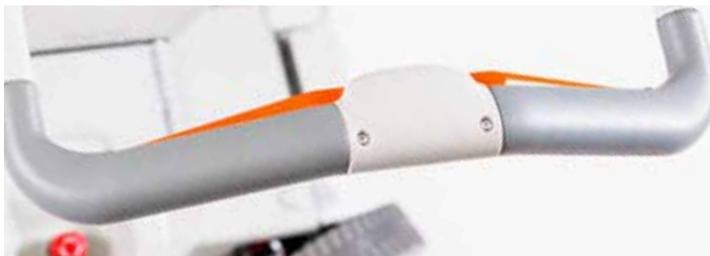
*The perceptive and ergonomic handle is equipped with load cells that intercepts your every move. By gently pushing it, EvaDrive moves forward. By pulling it lightly, EvaDrive reverses. The handle will sense your every desired movement. The EvaDrive will go in any direction at the point of your fingertips. The handle is ergonomic and adjustable in height. Also, a safety switch will prevent any undesired movement.*
